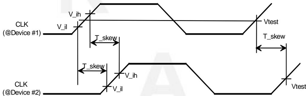
Figure 23: Clock Skew Diagram
