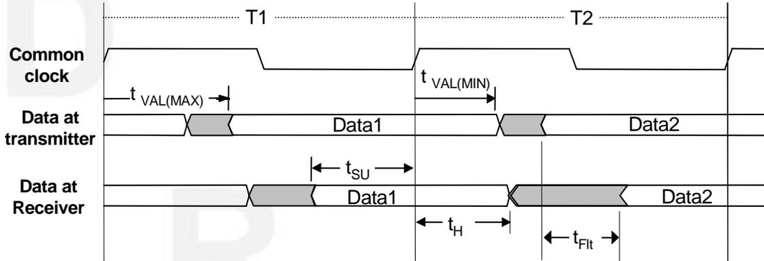
Figure 12: Common Clock Transfer Timings
