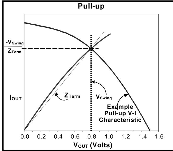
Figure 29: V/I Curve for AGP3.0 Transmitter Pull-up
