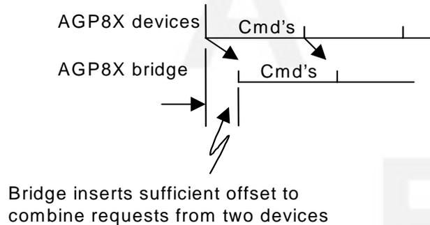
Figure 33: Potential Fan-Out Bridge Delays of Isochronous Periods for AGP3.0 Devices
