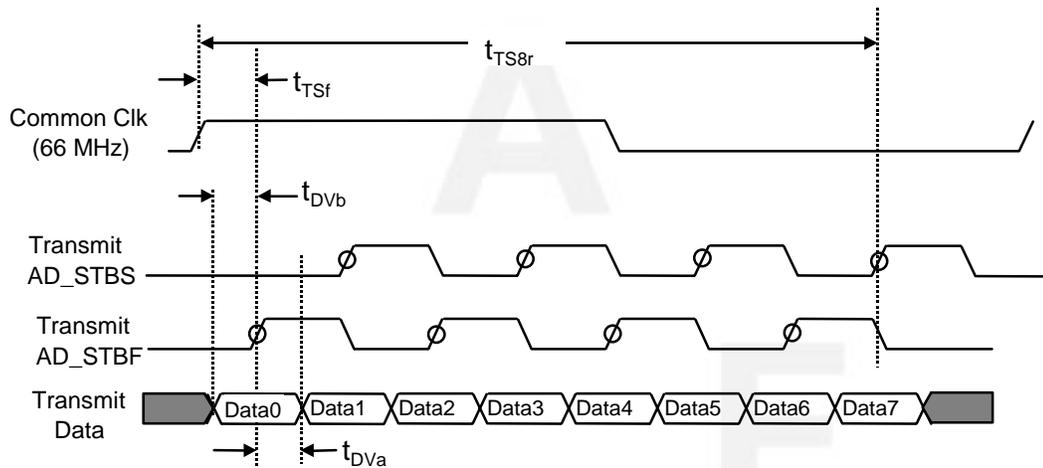
Figure 14: Transmit Strobe/Data Timing for 8X Source Synchronous Timing
