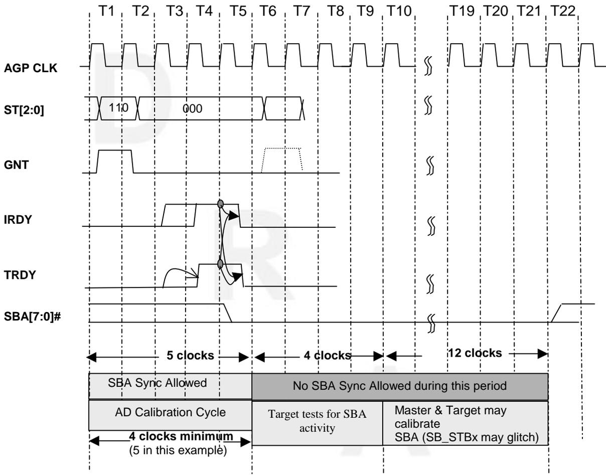
Figure 6: SBA Calibration When SBA Strokes are Stopped
