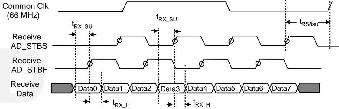
Figure 15: Receive Strobe/Data Timings for 8X Source Synchronous Timing
