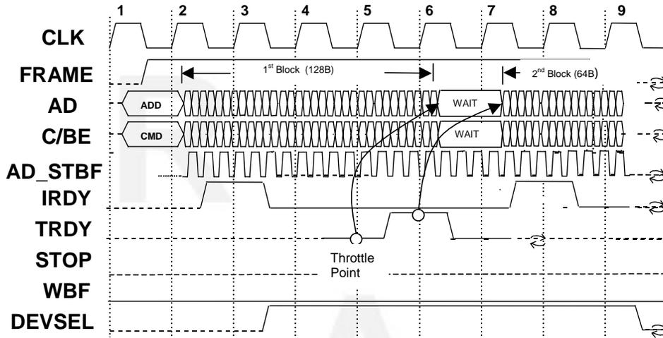
Figure 8: Fast-Write Showing Wait State Insertion
