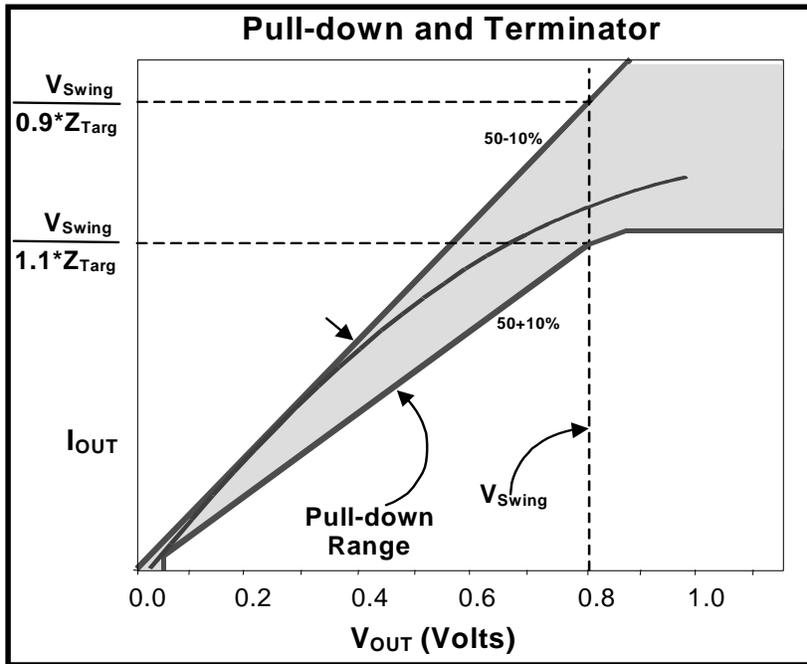
Figure 28: V/I Curve for AGP3.0 Receiver Termination Device
