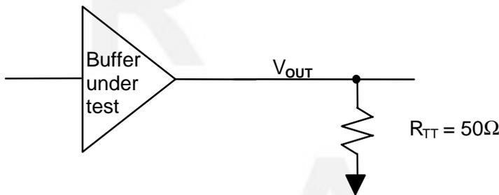
Figure 24: AGP3.0 Standard Buffer Test Load
