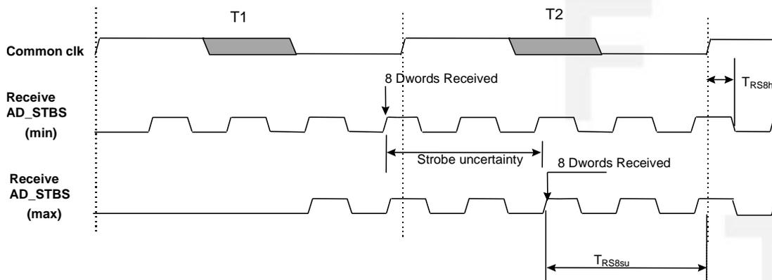
Figure 16: Minimum and Maximum Inner to Outer Loop Receive Timings
