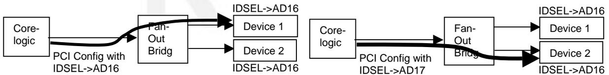
Figure 34: Fan-out Bridge Scheme Example
