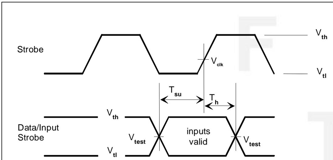
Figure 25: . Input Timing Measurement
