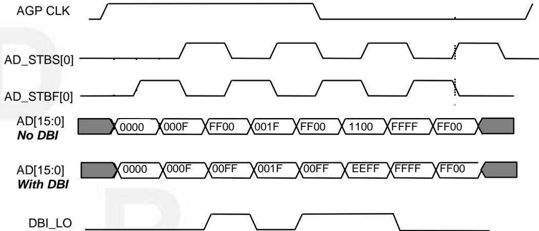
Figure 7: Usage of DBI on Source Synchronous Transfers
