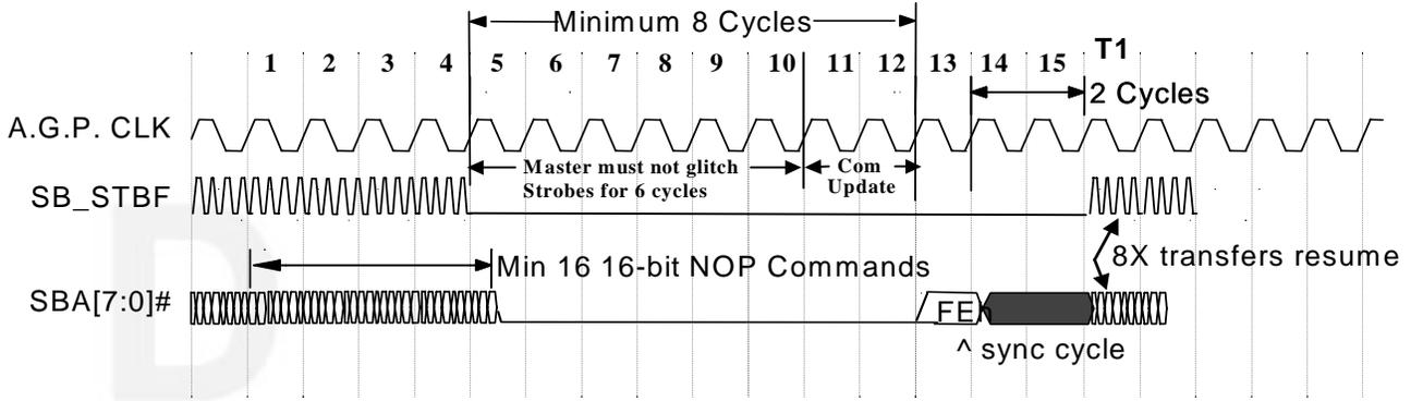
Figure 5: SB\_STB Stopping and Starting Sequence
