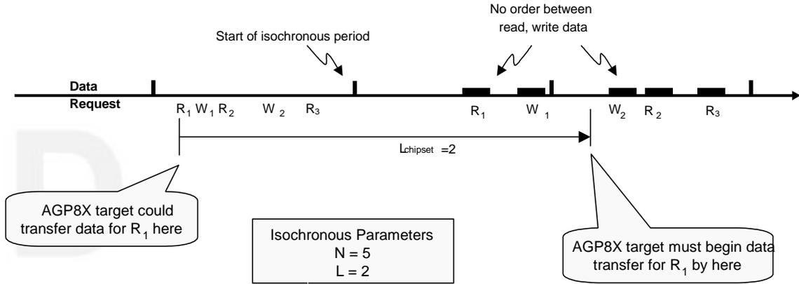
Figure 30: Isochronous Latency Determines Transfer Occurances
