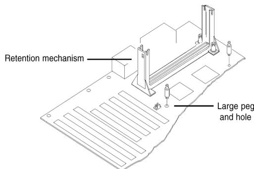
2. Slide a black plastic support onto each end of the fan or heatsink, making sure that the hole and clip are on the outside edge of the support. (If supports are reversed, the holes will not line up with the pegs on the motherboard.) Slide each support toward the center of the processor until the support is seated in the outside groove of the fan housing.
