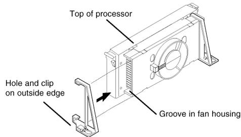
3. Slide the clip (A) on each support toward the processor, exposing the hole that will fit over the peg on the motherboard. Push the latches (B) on the processor toward the center of the processor until they click into place. (Refer to the figure below.)
