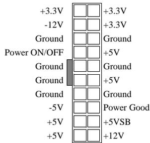
The ATX power supply has a single lead connector with a clip on one side of the plastic housing. There is only one way to plug the lead into the ATX power connector. Press the lead connector down until the clip snaps into place and secures the lead onto the connector.
