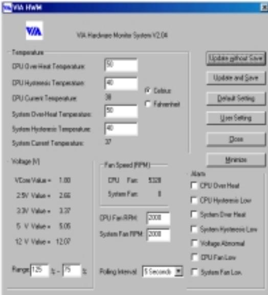
This screen shows the VIA hardware monitor system screen. It displays information about system temperature, voltages, and fan speed. Some items allow you to set the warning range; you can adjust your system settings to optimize values.
