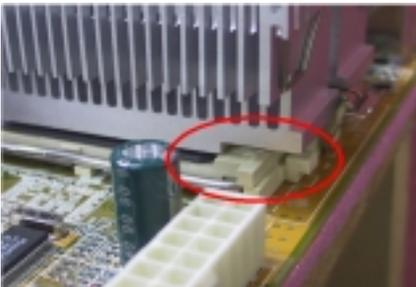
The left photo shows the bottom right side of the heatsink in contact with the right side of the Socket. In this situation, the processor die does not properly contact the heatsink. If you start the computer at this moment, it will immediately cause the processor damage. Always check this place when you finish the heatsink installation.
