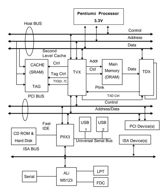
Fig. 1-2 System block diagram
