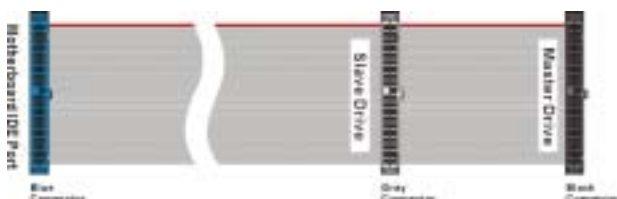
Figure 2-8. Ultra DMA 66 Ribbon Cable Outline
