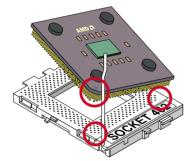
2 Take notice of the red circles as shown here. While inserting the CPU into the socket, you can find out there is a definite pin orientation for CPU and socket.
