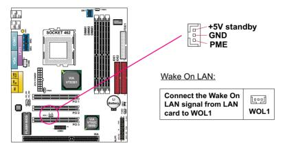
This connector is connected to the LAN card with a Wake On LAN output. The connector powers up the system when it receives a wake-up packet or signal through the LAN card.
