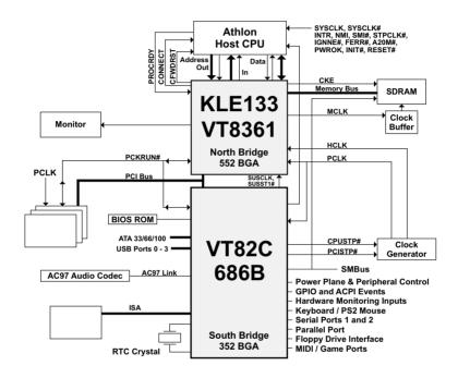
Diagram of KLE133 System Block with VT82C686B South Bridge
