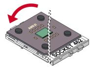
Make sure that the CPU is placed into the socket tightly. Then lower down the lever to complete the CPU installation.
