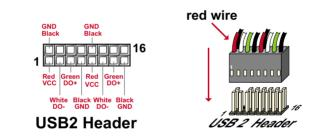
• When plugging the USB cable into USB2 Header, users must make sure the red wire is connected to the first pin.
