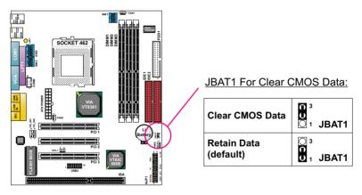
**NOTE:** You can clear CMOS by 2-3 pin closed when the system is POWER OFF. Then, return to 1-2 pin closed position (default). You may damage the mainboard if clearing the CMOS with POWER ON. Unplugging the power cord from power supply before clearing CMOS will be a safest bet for user.
