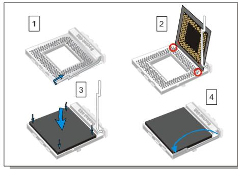
1. Lift the socket handle up to a vertical position.
