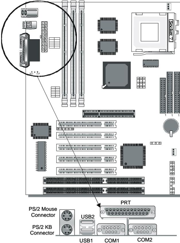
**1. Onboard Serial Port COM1,COM2**
