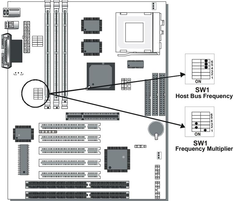
The SY-5EMA+ V1.0 Motherboard is designed to support most Pentium® class processors currently on the market. Jumpers SW1 is used to configure the Motherboard frequency parameters to match the working frequency of your CPU.
