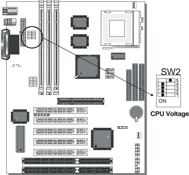
Please verify the correct voltage with your dealer before installation. Use the following tables to set SW2 to the proper "Voltage Value", according to the specifications marked on your CPU: This Motherboard comes with pre-configured setting of CPU voltage. However the voltage of your CPU maybe different with the default setting.
