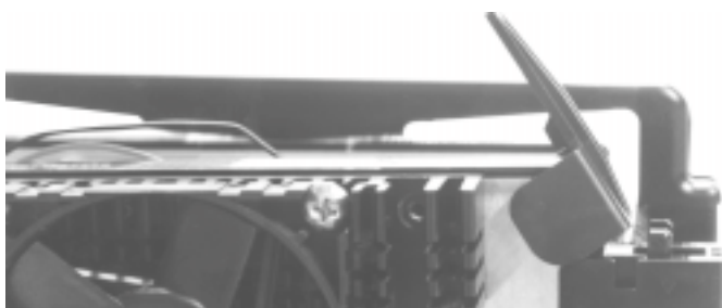
The processor raised out of the slot 2 connector by the reverse force of the lifters as they are pryed to a vertical position.
