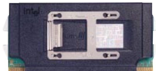
Example of an incorrectly installed retention clip
