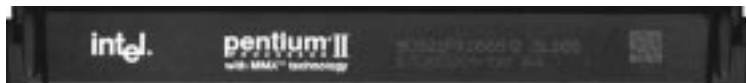
Intel Pentium II Processor in an SEC cartridge (233-450MHz 512KB/128KB/0KB L2 Cache)
