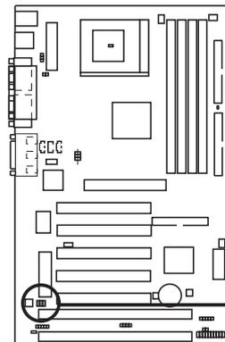
**NOTE:** Pin 3 is removed to ensure the correct orientation of the cable on it.
