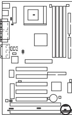
**TIP:** If the case-mounted LED does not light, try reversing the 2-pin plug.
