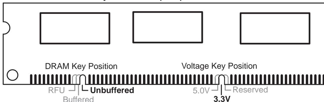
The notches on the DIMM module will shift between left, center, or right to identify the type and also to prevent the wrong type from being inserted into the DIMM slot on the motherboard. You must ask your retailer the correct DIMM type before purchasing. This motherboard supports four clock signals.
