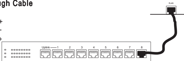
P2B-L/S/LS Typical Network Connection
