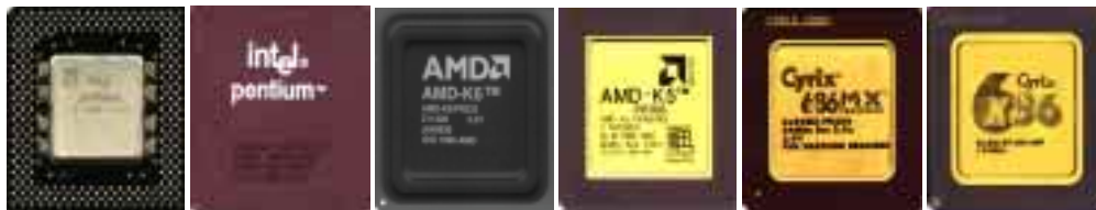
Pentium MMX (P55C) (150MHz-233MHz) Intel Pentium (P54C) (75MHz-200MHz) AMD-K6 (PR166 and faster) AMD-K5 (PR75-PR133) IBM/Cyrix 6x86(MX) (PR166 and faster) IBM/Cyrix 6x86(M1) (PR166 and faster)
